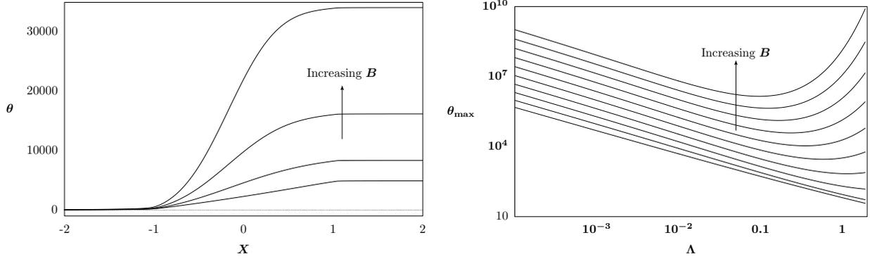
Figure 8: (left) Scaled temperature profiles for  $\Lambda = 0.01$ ,  $Pe = 10$  and  $B = 0, 1, 2, 3$ . (right) Maximum scaled temperature as a function of  $\Lambda$ :  $\theta_{\max} = O(\Lambda^{-1})$  for  $B = 0$  (solid curve).
