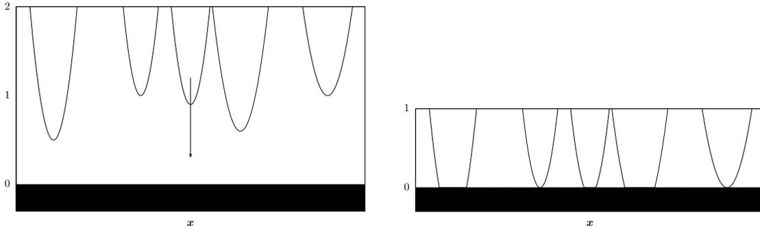
Figure 2: Schematic representations of the the wafer surface (solid black),  $z = 0$ , and the asperities on the pad surface (upper surface): (left) being brought into contact, (right) in contact, with some asperity tips being deformed.
