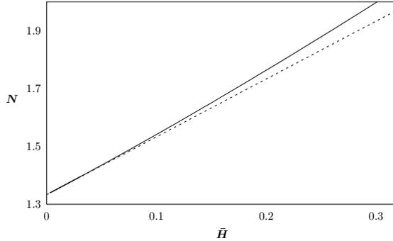
Figure 5: The near-linear relation between average gap height and applied load at fixed  $\delta$ : solid curve - numerical results, dashed curve - linear behavior for  $\bar{H} \rightarrow 0$ , equation (19).
