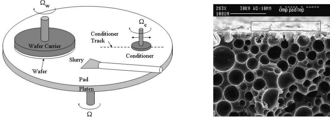
Figure 1: (Left) Schematic of a typical single-wafer rotary CMP tool. (Right) Scanning Electron Micrograph cross-section of a used, conditioned void-filled polyurethane polishing pad. Surface asperities can be seen in the boxed region at the top of the image. The scale bar at the top center is 100 microns (0.1 mm) long. Voids average about 30 microns in diameter and occupy about 60% of a planar cross-section (Data by Letitia Malina, Motorola).
