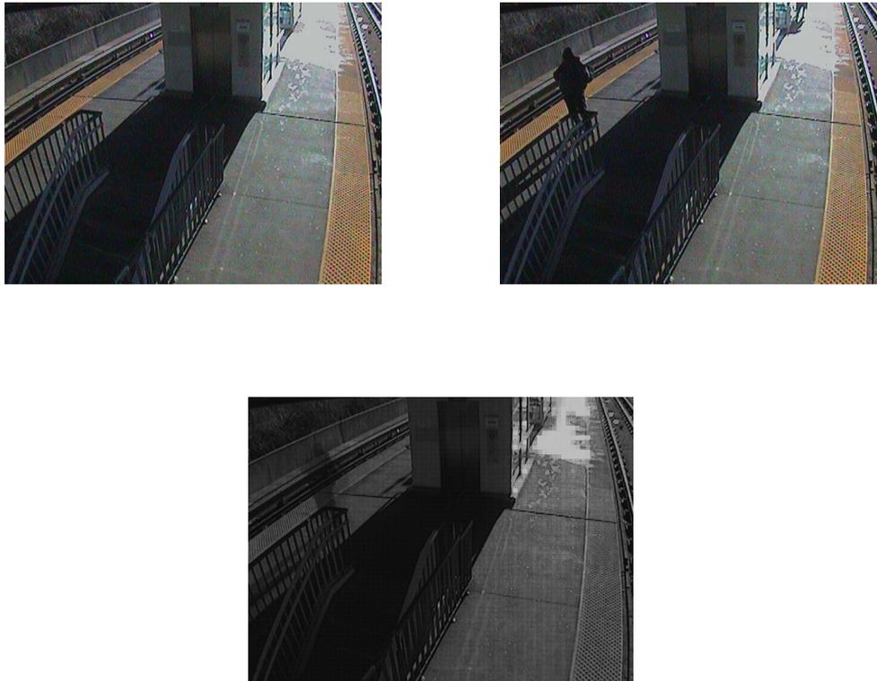
Figure 1: An empty scene (top left) shows the full background image of a train platform. After some time, a person enters the scene, walks around and eventually stands still on the platform (top right). The algorithm of computing the partial background average (9) recognises the person. However, when the person remains static for a period of time, their outline become part of the background (bottom, in greyscale).
