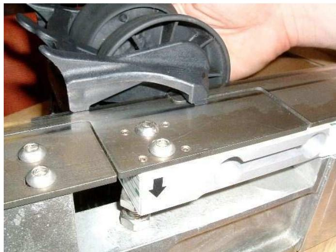
*Figure 3.* A loadcell with the steel plate on top, and a (handheld) carrier moving over it from right to left. Note the two tracks worn into the steel plates by the moving contact points of the carrier.
