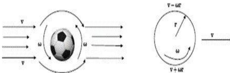
Figure 1: Velocity of a soccer ball.
