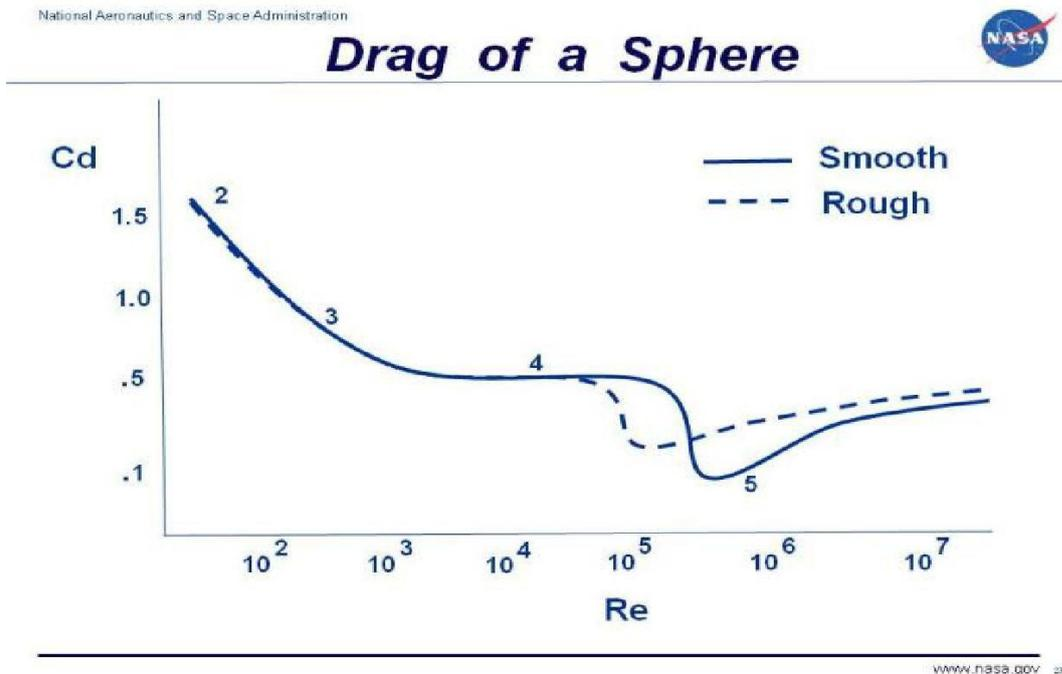
Figure 3: Drag coefficient for rough and smooth spheres.
