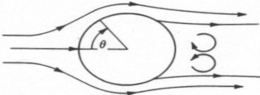
Figure 2: The general character of flow over a cylinder at high Reynolds numbers.
