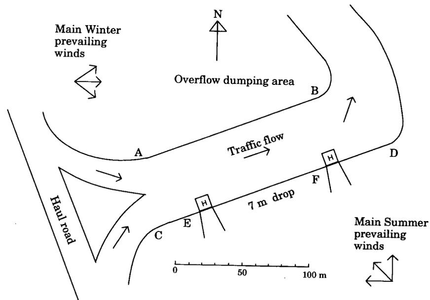
Figure 1: Ground plan of the dumping site at Warkworth's Singleton mine. The two squares labelled H represent the dumping hoppers.
