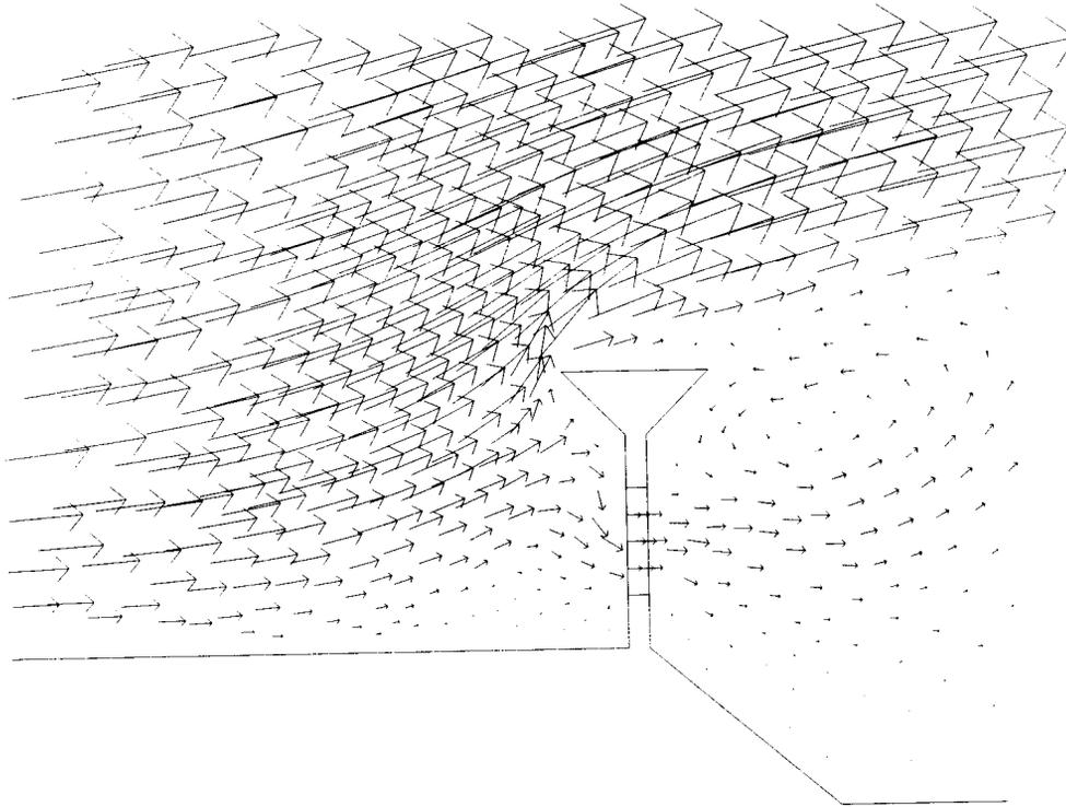
Figure 4: Air velocity around a barrier with an angled overhang and a porous lower section.
