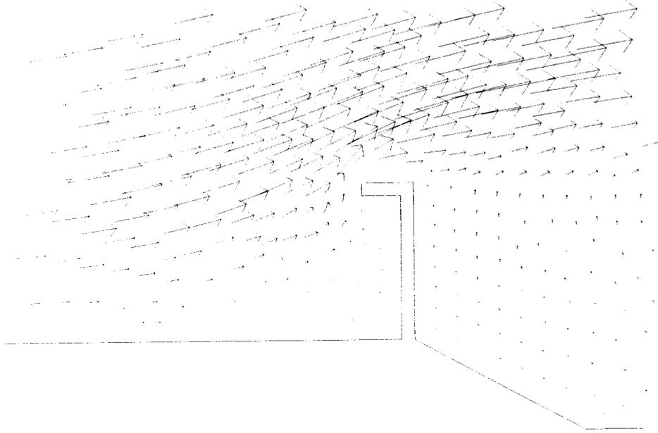
Figure 2: Air velocity in the vicinity of a solid barrier with a right-angle overhang. The length of each arrow is proportional to the local velocity.
