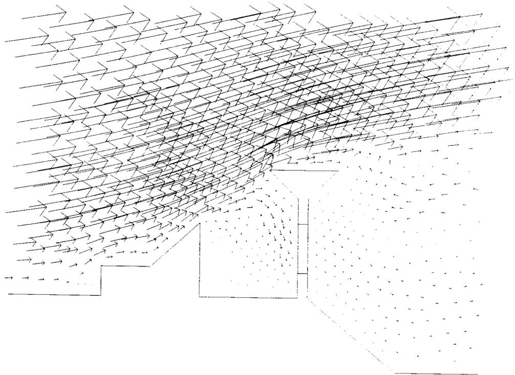
Figure 5: Air velocity over a two-dimensional truck in front of a barrier with an angled over-hang and a porous lower section.
