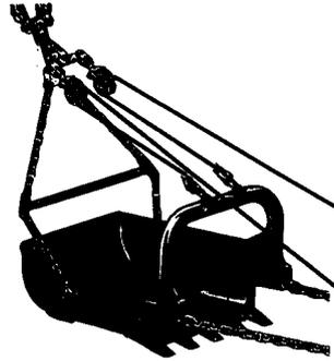
Figure 2: An actual bucket is pictured as it is lowered to the ground in preparation for dragging.
