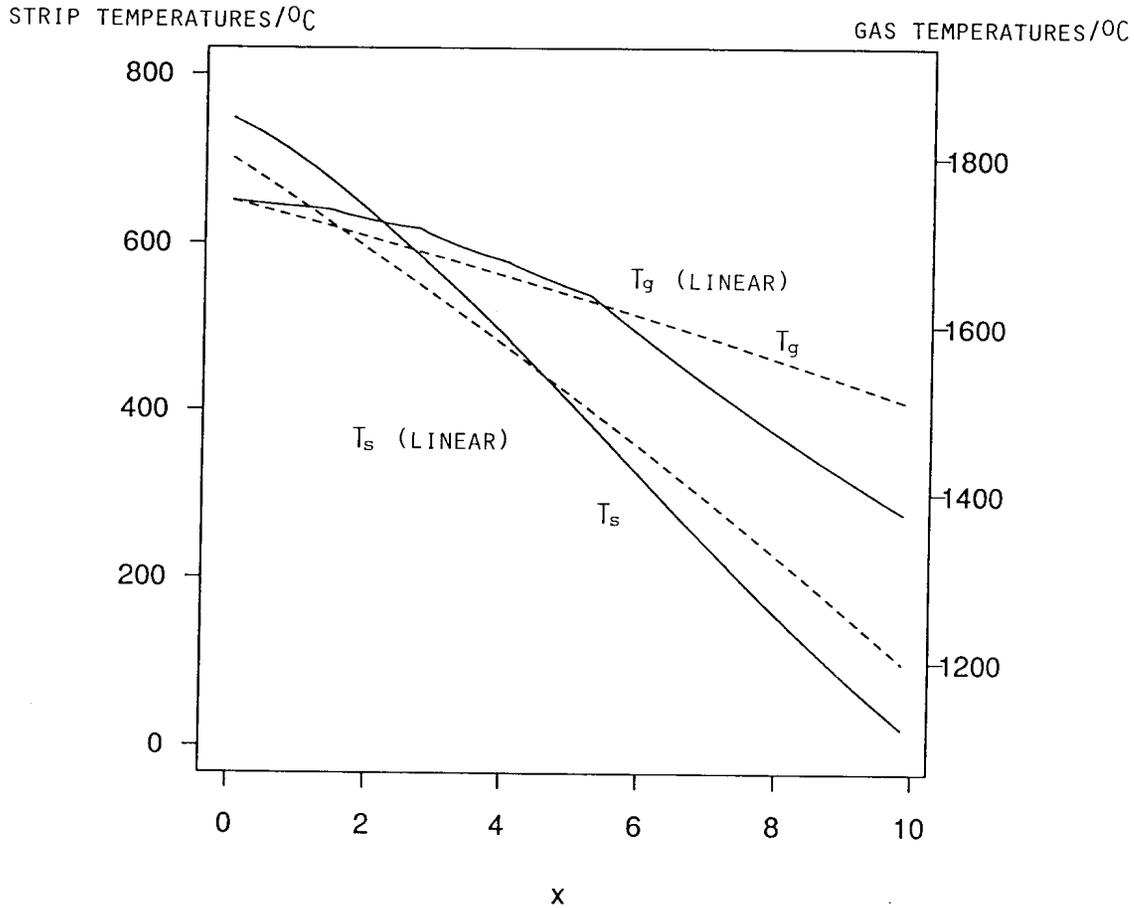
Figure 2: Strip and gas temperatures from steady state model (solid lines) and linearised model (dashed lines). Note the two different axes.
