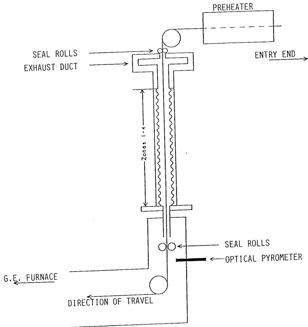
Figure 1: Cross-section through a Selsas furnace.
