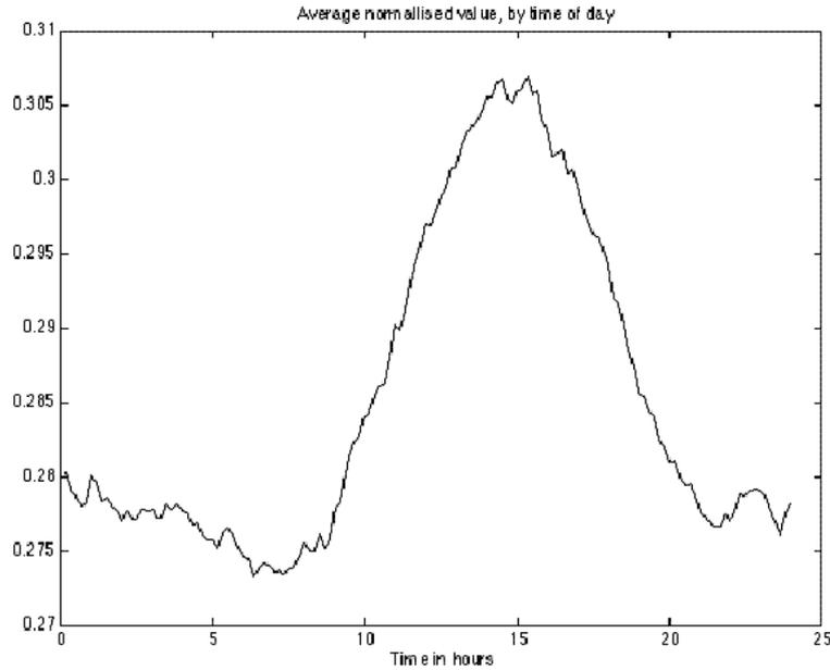
Figure 5. Average daily normalised wind speed for wind farm data.
