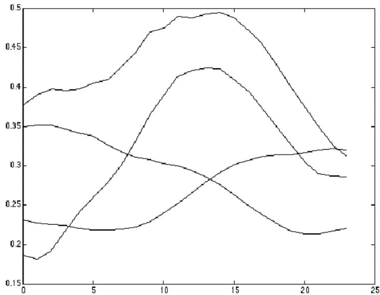
*Figure 7.* mean values for four clusters that give different daily wind profiles.
