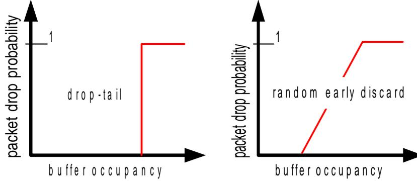
Figure 3: Packet loss probability for the two packet discard policies.
