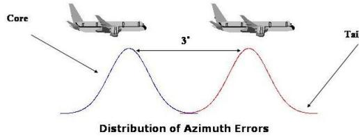
Figure 3: Horizontal overlap convolution
