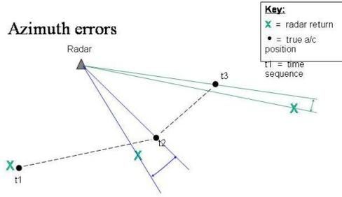
Figure 1: Determining azimuthal error
