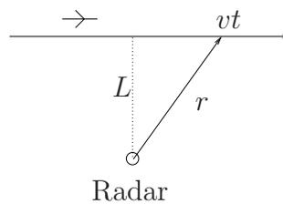
Figure 7: Calculating range on a fly-by
