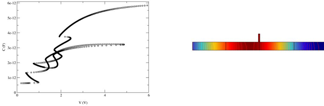
Figure 3: Calculated capacitance-voltage ( $C - V$ ) characteristic (left) of the 'see-saw' RF MEMS switch shown on the right. Only 1/2 of the total switch is shown.
