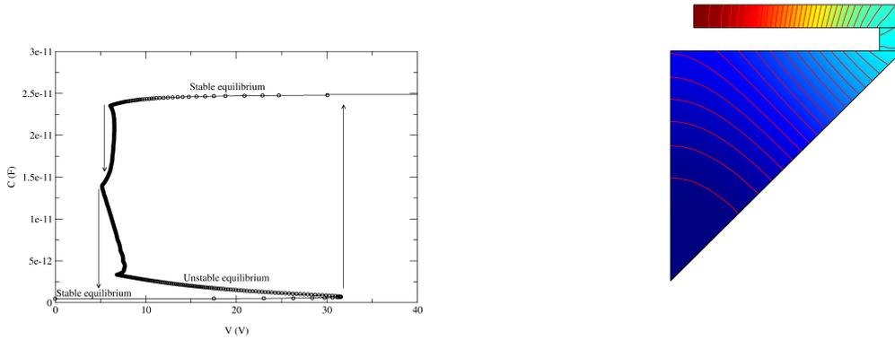
Figure 2: Calculated capacitance-voltage ( $C - V$ ) characteristic (left) of the RF MEMS switch shown on the right (which is similar to that in figure 1(b)). Only 1/8 of the total switch is shown. The color indicates the height, anchor is red, dielectric height is blue. Arrows indicate discontinuities that occur under voltage controlled actuation.
