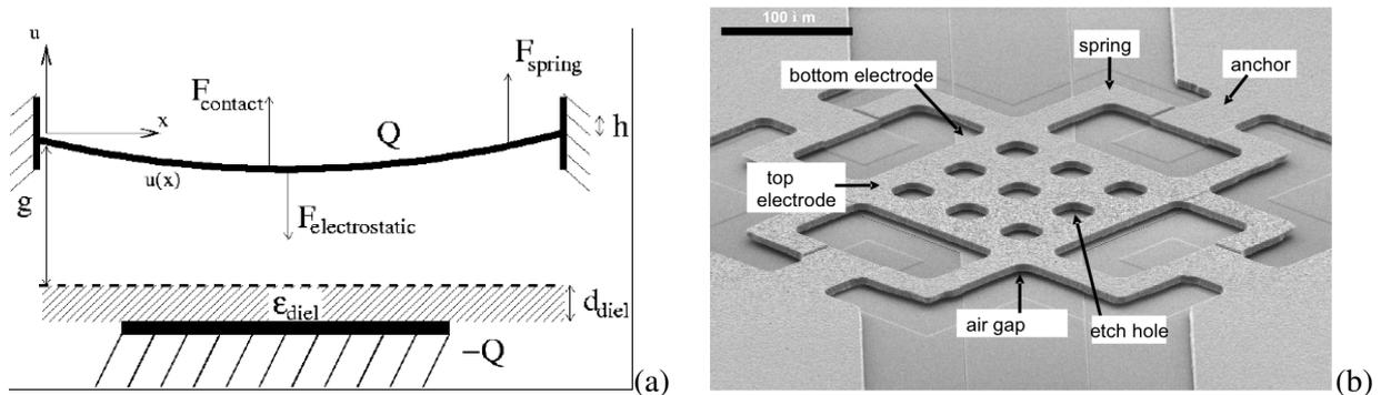
Figure 1: (a) Schematic cross-section of a capacitive RF MEMS switch. (b) Scanning electron microscope picture of a capacitive RF MEMS switch.
